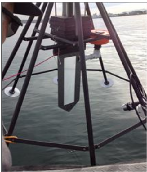
Figure 3. Passive Push sampler frame with polyethylene passive sampler, mounted in deployment system with attached timed-release recovery buoy (SPAWAR Systems Center Pacific, 2018).
