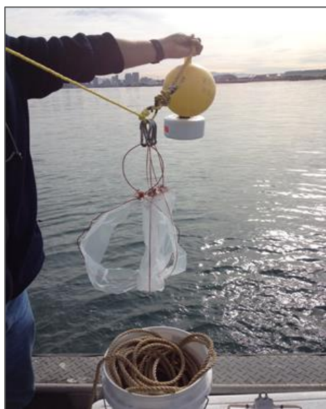
Figure 4. PE passive samplers for water column sampling (Southern California Coastal Water Research Program, 2018).
